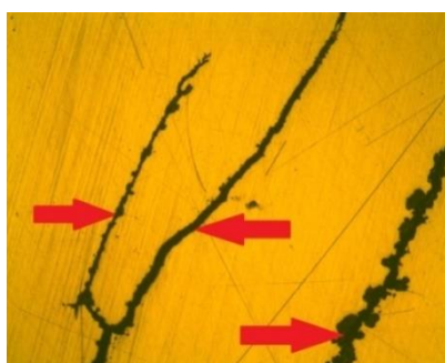
Fig. 5. Metal structure of a defective rail T VI 08 60E1 at x50 magnification
